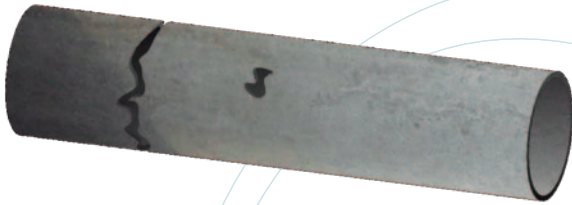
Crack or burst or deteriorated pipe wall
